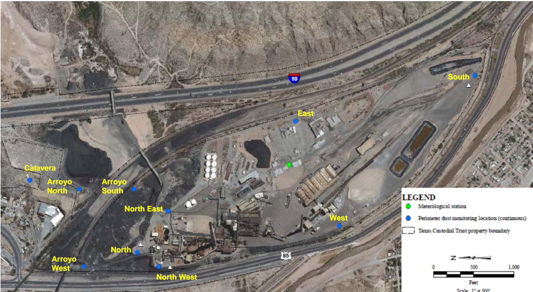
Figure 1 Texas Custodial Trust Former Asarco Smelter Site El Paso, Texas Dust Monitoring Locations
