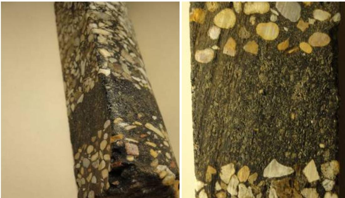
**Figure 4. Slag in Old HMA Cores from the Bryan District.**
