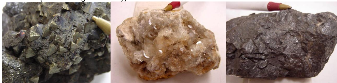
Figure 6. Zinc minerals (left to right, sphalerite, smithsonite, and wurtzite). (U.S. Geological Survey)
